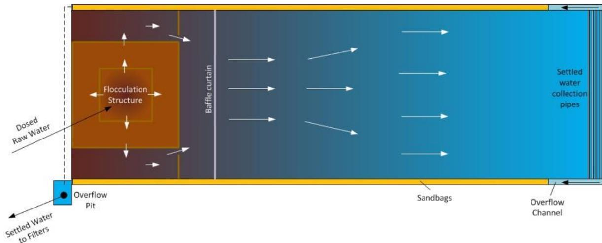
Figure 3: Poolifier schematic showing flocculation structure and flow path.
