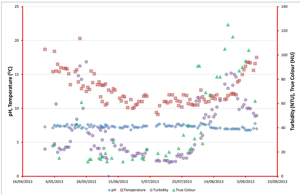
Figure 6: Swan Hill WTP raw water during continuous Poolifier operation (30th April to 9th September 2013).
